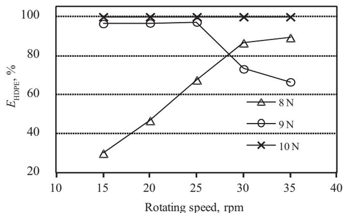
Fig. 3. The influence of rotating speed of the separating system on the effectiveness of separation of HDPE from a HDPE/PET/PVC mixture ( $E_{HDPE}$ )
