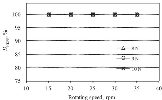
Fig. 2. The influence of rotating speed of the separating system on the accuracy of separation of HDPE from a HDPE/PET/PVC mixture ( $D_{HDPE}$ )
