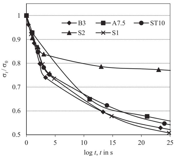
Fig. 3. The effect of time ( $t$ ) on normalized stress ( $\sigma_t/\sigma^*$ ) of XNBR vulcanizates at strain of 200 or 300 % at the room temperature
