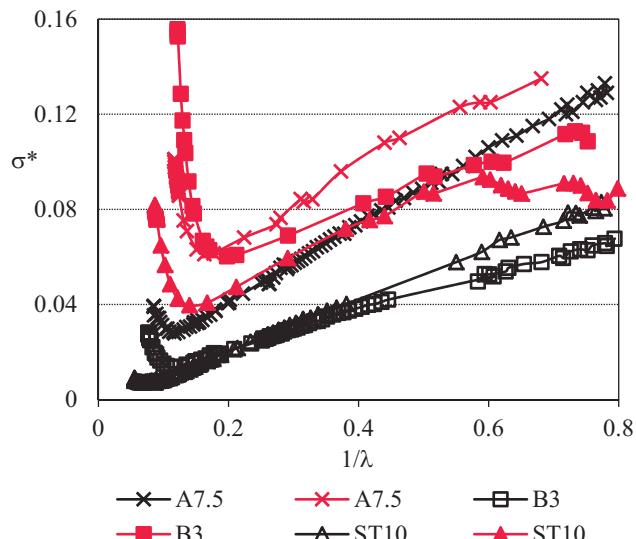
Fig. 2. The effect of inverse extension ratio ( $1/\lambda$ ) on reduced stress ( $\sigma^*$ ) of XNBR vulcanizates deformed at different rates, crosshead speed equal to 25 mm/min (black curves) and 1000 mm/min (red curves), respectively
