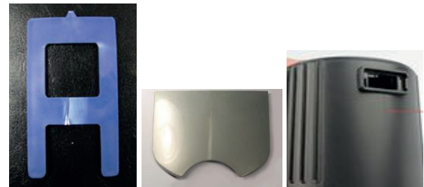
Fig. 5. Examples of injection molded parts with visible weld lines [13–15]
