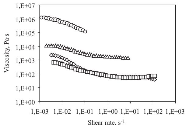
**Fig. 1.** Viscosity curves determined at 130 °C for CTP-polymer compositions:  $\diamond$  — CTP,  $\square$  — CTP+25 wt % PET,  $\circ$  — CTP+25 wt % UP,  $\triangle$  — CTP+10 wt % PC
