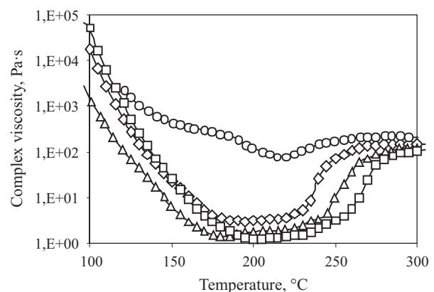
**Fig. 2.** The plots of complex viscosity versus temperature determined for CTP-polymer compositions:  $\diamond$  — CTP,  $\square$  — CTP+10 wt % PET,  $\circ$  — CTP+10 wt % UP,  $\triangle$  — CTP+10 wt % PC
