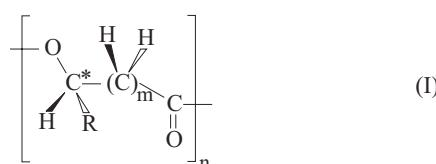
where: m – the number of carbon atoms in the backbone of the PHA building blocks, n – the degree of polymerization (numbers of monomers in polyester chain), R – the side chain of the building blocks.
