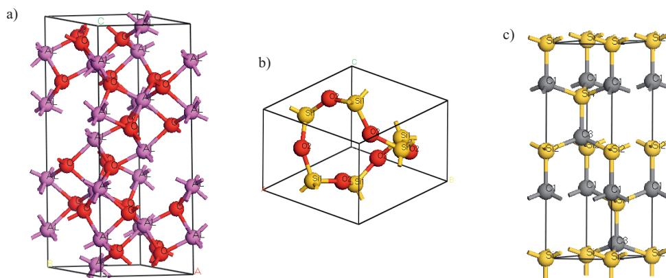
Fig. 1. Ceramic crystal structures of: a)  $\text{Al}_2\text{O}_3$ , b)  $\text{SiO}_2$ , c)  $\text{SiC}$
