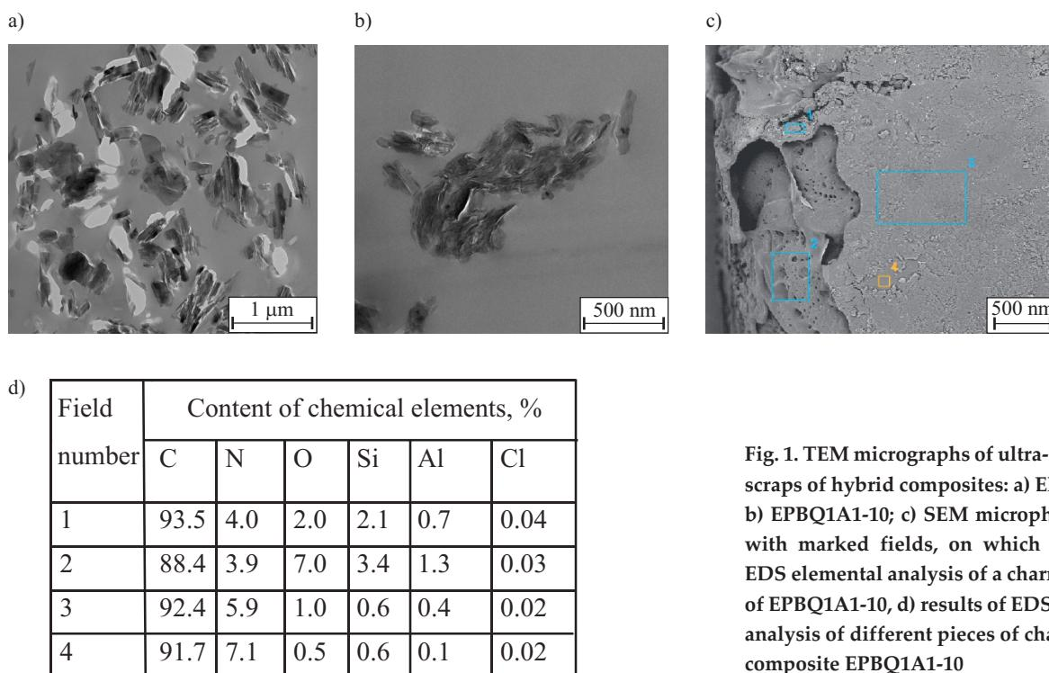
**Fig. 1.** TEM micrographs of ultra-microtome scraps of hybrid composites: a) EPBQ1A1-5, b) EPBQ1A1-10; c) SEM microphotography with marked fields, on which was made EDS elemental analysis of a charred sample of EPBQ1A1-10, d) results of EDS elemental analysis of different pieces of char of tested composite EPBQ1A1-10
