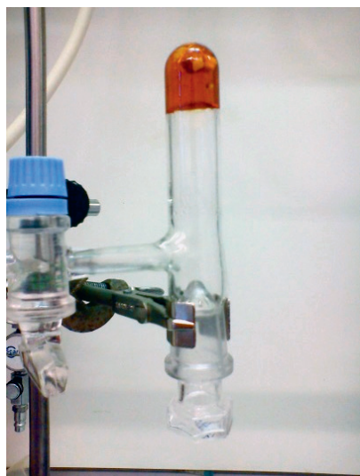
Fig. 5. Reaction product from AcGGM-Br initiated GMA graft polymerization at 80 % conversion. [GMA]_0/[AcGGM-Br]_0/[Me_6-TREN]_0 = 200/1/0.2
