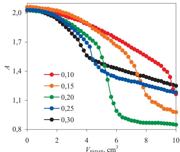
Fig. 7. Spectrophotometric reverse titration curves obtained for different PHMB mers concentrations (given in mmol/dm<sup>3</sup>) in the analyzed solution using the dye solution with constant concentration
