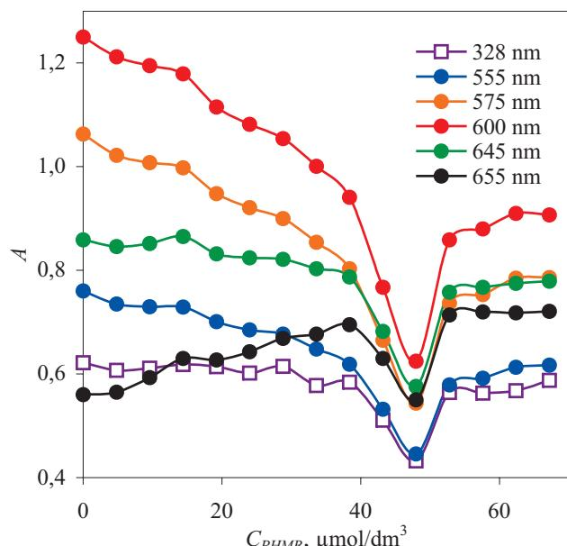
Fig. 3. Dependences of absorbance (A) determined at various wavelengths on PHMB mers concentration ( $C_{PPHMB}$ ) in solutions containing  $25 \mu\text{mol}/\text{dm}^3$  of NBB dye
