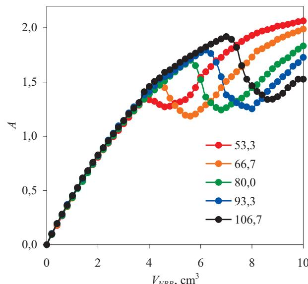
Fig. 4. Spectrophotometric direct titration curves obtained for different PHMB mers concentrations (given in  $\mu\text{mol}/\text{dm}^3$ ) in the analyzed solution using the dye solution with constant concentration
