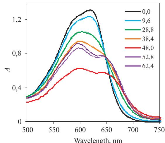
Fig. 1. UV-Vis spectra of NBB-PHMB mixtures obtained for 25 µmol/dm<sup>3</sup> solution of NBB and the indicated PHMB concentrations (given in µmol/dm<sup>3</sup> of mers)
