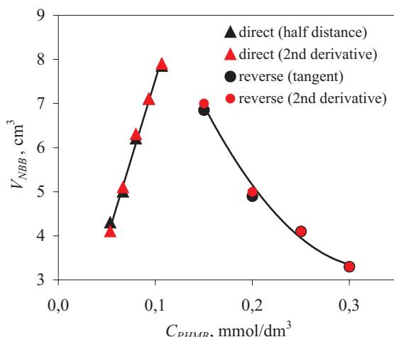
Fig. 6. Dependence between PHMB mers concentration and titrant volume at the endpoint for direct and inverse titration
