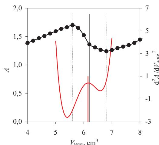
Fig. 5. The illustration of graphic methods of endpoint determination for direct titration (black lines – half distance method, red lines – second derivative method)
