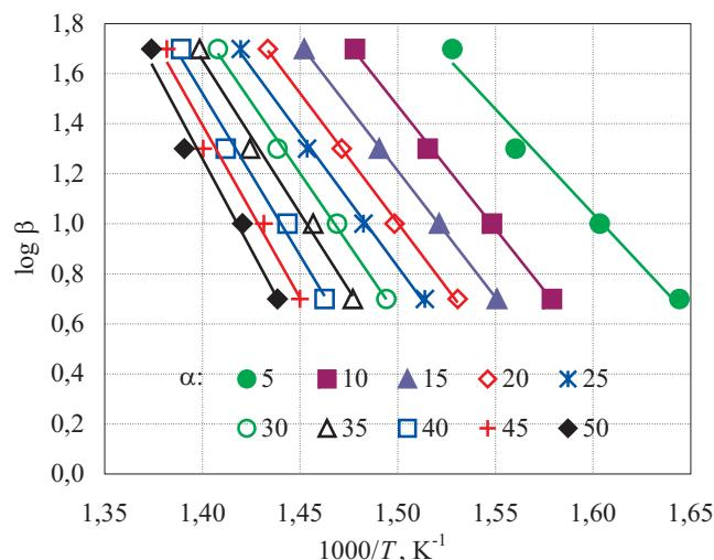
Fig. 2. Plots for determination of activation energy of thermal decomposition by Ozawa method for various decomposition rates of isocyanate-epoxy system without EMI at various heating rates
