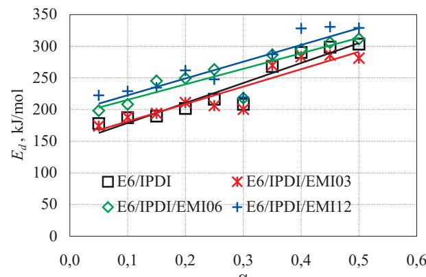
**Fig. 4.** Activation energy ( $E_d$ ) values determined by Friedman method versus conversion rate ( $\alpha$ ) for isocyanate-epoxy system with various EMI content
