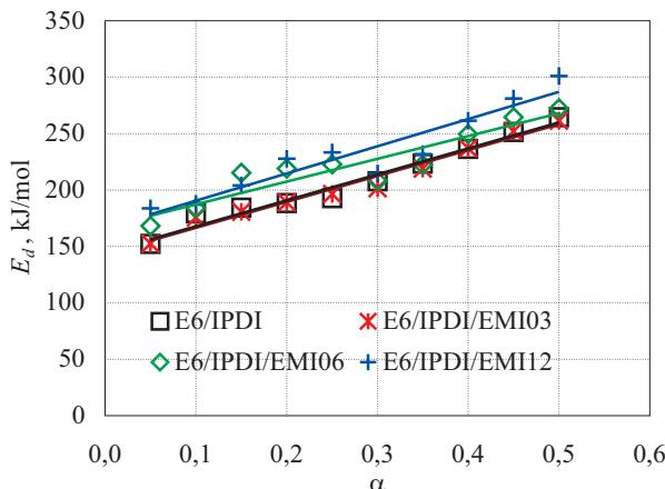
Fig. 3. Activation energies ( $E_d$ ) determined by Ozawa method versus conversion rate ( $\alpha$ ) for isocyanate-epoxy system with various EMI content
