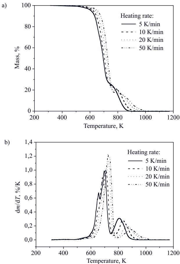
**Fig. 1. TG (a) and DTG (b) curves for isocyanate-epoxy system obtained at various heating rates**
