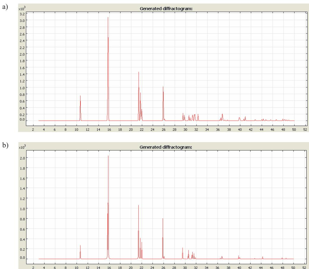
Fig. 4. Comparison of the reference diffraction pattern (a) with diffraction pattern found by CrystalFinder as the best fit individual (b)
