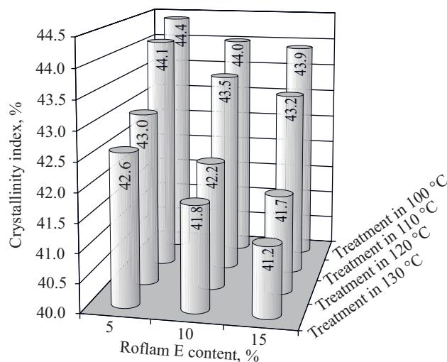
**Fig. 2.** Changes of crystallinity index of modified flame retardant PET fibers, evaluated on the basis of DSC measurements, as a function of Roflam E content and the temperature of modifying bath
