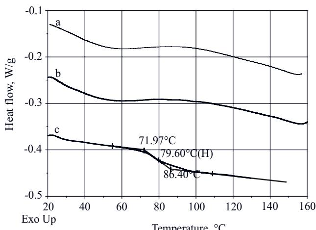
Fig. 5. An example of a setting-up of DSC curves registered for: a) modified flame retardant PET fibers (15 % Roflam E, in bath of temperature 130 °C) directly after the formation process, b) the same fibers after 5 years of natural ageing, c) the material of these fibers earlier quenched from the melt; heating rate 10 °C/min, atmosphere N<sub>2</sub>, flow 40 cm<sup>3</sup>/min; analysis of the glass transition region
