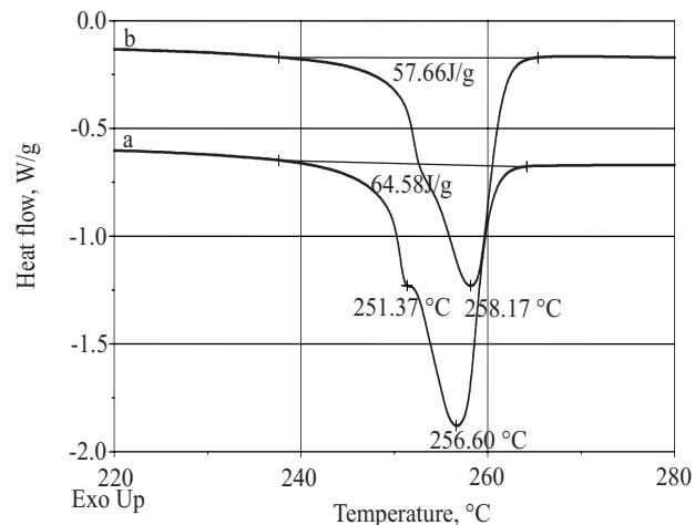
Fig. 6. DSC curves of flame retardant PET fibers modified with 15 % Roflam E in bath of temperature 130 °C: a) after 5 years of ageing in atmospheric conditions, b) directly after the fabrication; heating rate 10 °C/min, atmosphere N<sub>2</sub>, flow 40 cm<sup>3</sup>/min; analysis of the melting region
