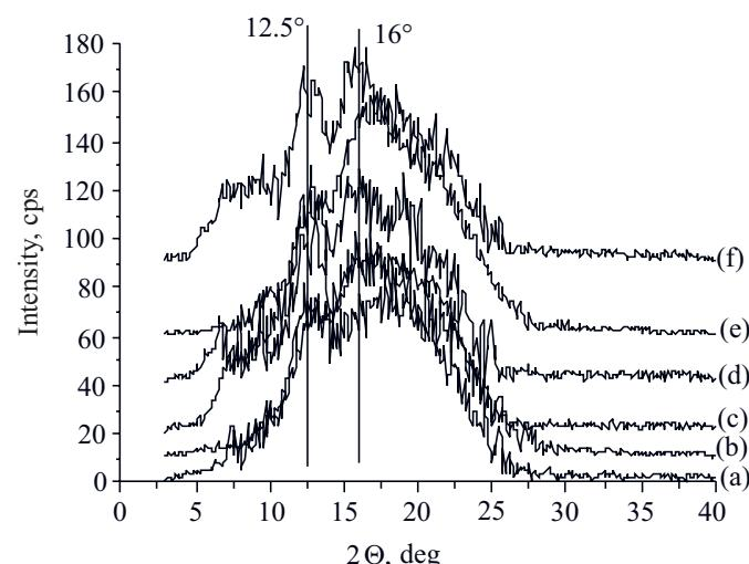
Fig. 7. WAXS patterns of terpolymer SMP material before and during the degradation process respectively: (a) — before degradation, (b) — after 2 weeks, (c) — after 4 weeks, (d) — after 6 weeks, (e) — after 8 weeks, (f) — after 10 weeks of degradation
