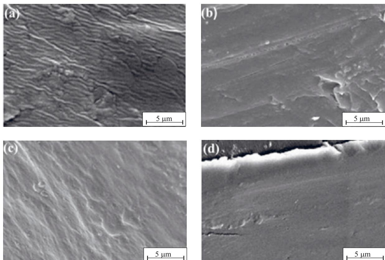
Fig. 1. SEM microphotographs of degraded staple samples, degradation respectively: (a) — 2 weeks, (b) — 4 weeks, (c) — 8 weeks and (d) — 10 weeks
