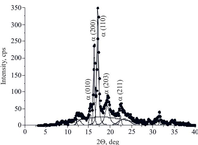
Fig. 10. WAXS pattern of sample subjected to degradation for 18 weeks
