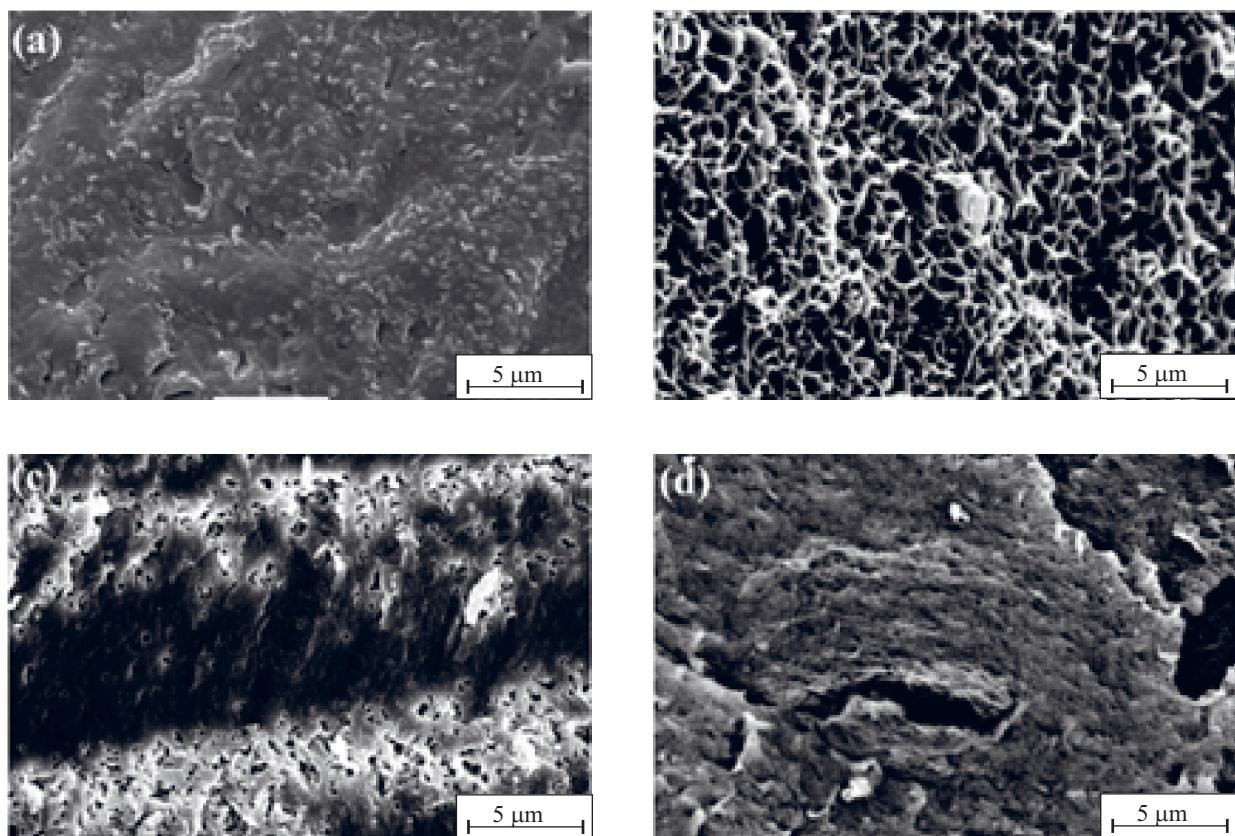
Fig. 2. SEM microphotographs of degraded staple samples, degradation respectively: (a) — 12 weeks, (b) — 14 weeks, (c) — 16 weeks and (d) — 18 weeks
