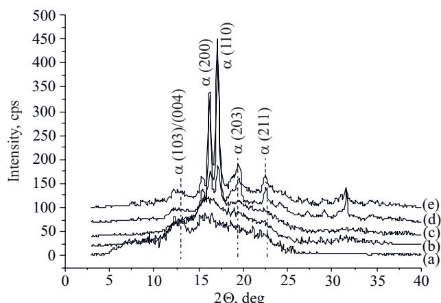
Fig. 8. WAXS diffraction patterns of staples during the degradation process: (a) – after 10 weeks, (b) – after 12 weeks, (c) – after 14 weeks, (d) – after 16 weeks, (e) – after 18 weeks of degradation
