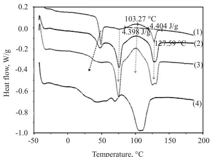
Fig. 4. DSC curves of samples: (1) — before degradation, (2) — after 8 weeks, (3) — after 10 weeks, (4) — after 18 weeks of degradation
