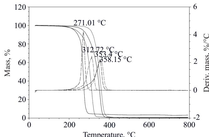
Fig. 6. TG and DTG curves of material before and during the degradation process for 12–18 weeks
