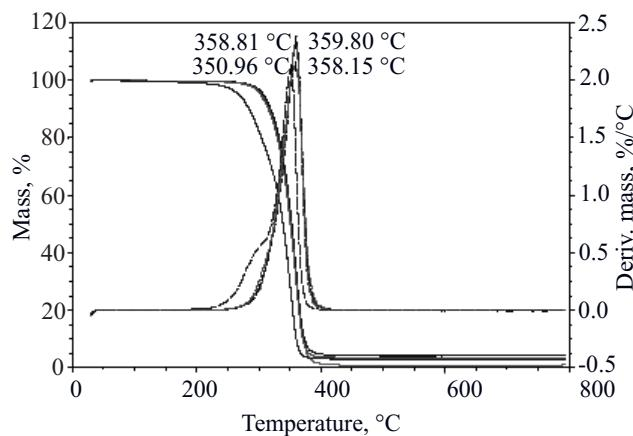
Fig. 5. TG and DTG curves of material before and during the degradation process for 4–10 weeks
