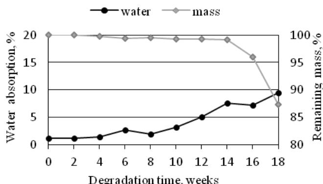
Fig. 3. Changes of sample mass during degradation and changes of water sorption
