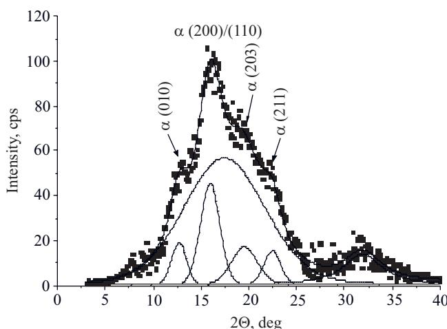
Fig. 9. WAXS pattern of sample subjected to degradation for 12 weeks
