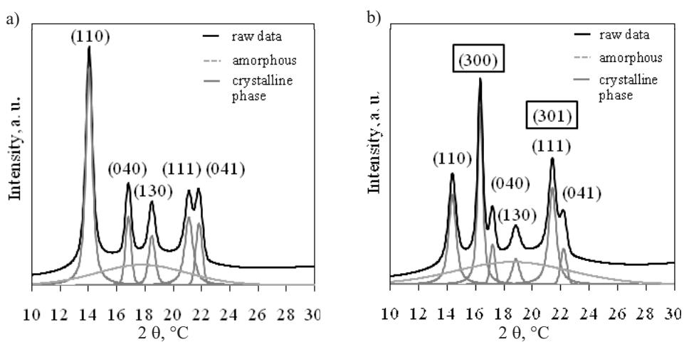
Fig. 3. WAXS patterns of isotactic polypropylene with separation of maxima: a) isotactic polypropylene without silver nanoparticles, b) composite containing 0.4 wt % nAg
