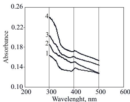
Fig. 2. UV/VIS spectra for isotactic polypropylene composites containing silver nanoparticles: 1 – 0.1 wt % nAg, 2 – 0.2 wt % nAg, 3 – 0.4 wt % nAg, 4 – 0.6 wt % nAg
