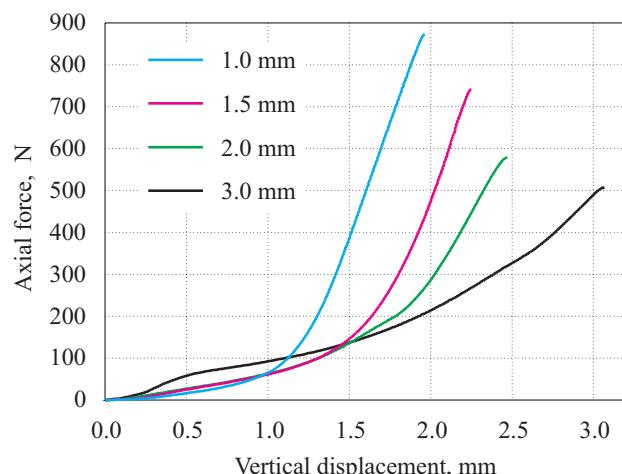
**Fig. 4.** The influence of vertical displacement during moving between the threaded connection elements on the axial force for different thicknesses of sealing insert (exemplary courses)
