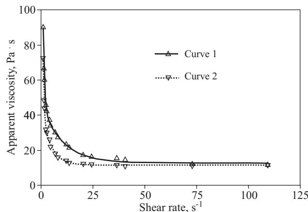
Fig. 1. Changes in apparent viscosity of EPBP1K-3.0 composite at increasing (curve 1) and decreasing (curve 2) shear rate
