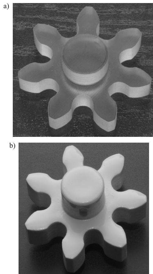
Fig. 2. View of gear wheel prototypes made of: a) unfilled EP, b) EPBP1K-3.0
