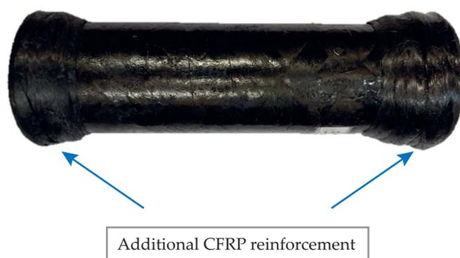
**Fig. 3. FW pipe with additional reinforcement prepared for axial compression test**
