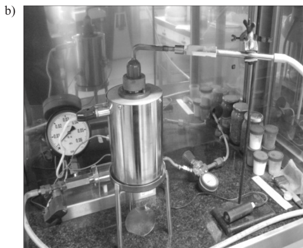
Fig. 1. Test stand for determination of minimum ignition temperature for: a) dust layer, b) dust cloud
