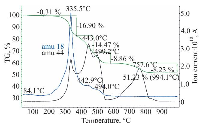
Fig. 4. Temperature-dependent mass change (TG) and results of mass spectroscopy (ion current for mass numbers 18 and 44)
