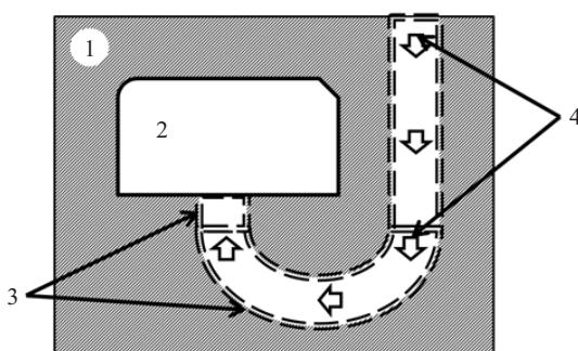
Fig. 1. A simplified diagram of the technology for producing large iron casts, where: 1 – sand mould, 2 – mould cavity, 3 – EG Runner gating system, 4 – direction of liquid metal flow
