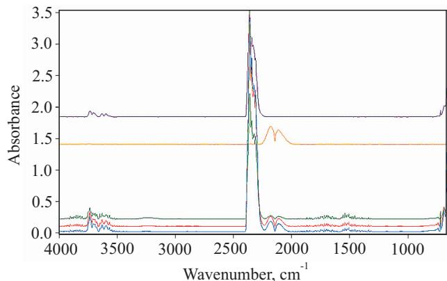
Fig. 14. Comparison of the extracted IR-spectra at 446 °C (blue), 495 °C (red) and 795 °C (green) with the library spectra of CO<sub>2</sub> (purple) and CO (orange)
