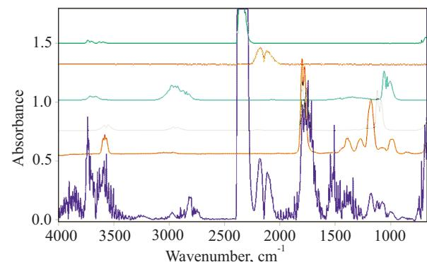
Fig. 12. Comparison of the extracted IR-spectrum at 340 °C (blue) with the library spectra of CO (red), CO<sub>2</sub> (green), acetic acid (orange), formic acid (purple) and methanol (turquoise)
