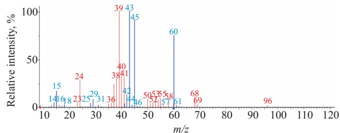
Fig. 7. Mass spectrum of the cellulose sample measured at 335 °C (red) in comparison with the NIST literature spectrum of acetic acid ( $C_2H_4O_2$ , blue)
