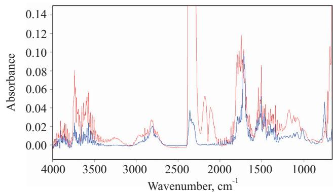
Fig. 13. Comparison of the extracted IR-spectrum at 340 °C (red) with the extracted spectrum of fructose (blue)
