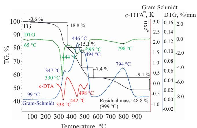
Fig. 8. TG- (black), DTG- (green) Gram-Schmidt- (blue) and c-DTA-results (red) of the sample
