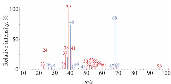
Fig. 6. Mass spectrum of the cellulose sample measured at 335 °C (red) in comparison with the NIST literature spectrum of 3-methyl-2,5-furandione ( $C_5H_4O_3$ , blue)
