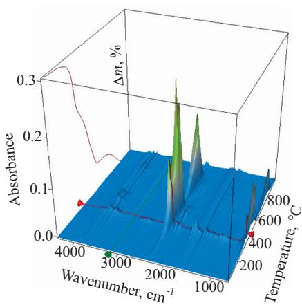
Fig. 9. 3D view of all detected IR-spectra versus temperature including the TG results at the side face
