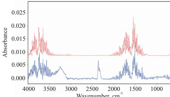
Fig. 11. Comparison of the extracted IR-spectrum at 74 °C (blue) with the library spectrum of water (red)
