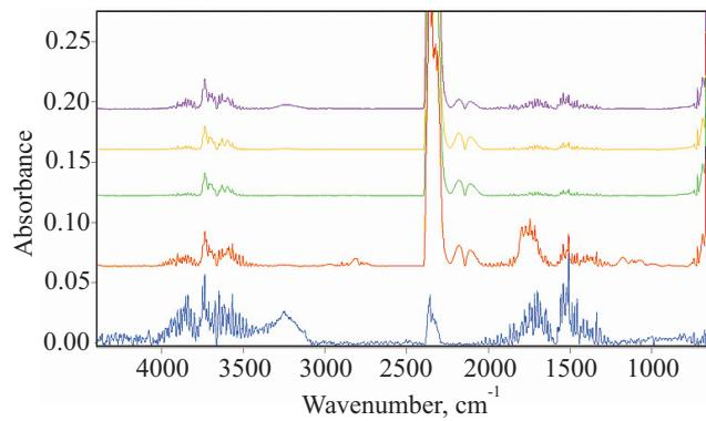
Fig. 10. Extracted IR spectra of the specimen at 74 °C (blue), 340 °C (red), 446 °C (green), 495 °C (orange) and 795 °C (purple)
