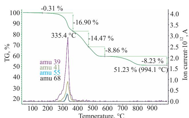
Fig. 5. Temperature-dependent mass change (TG) and results of mass spectroscopy (ion current for mass numbers 39, 41, 55 and 68)
