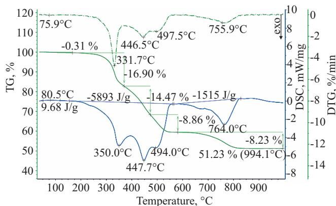
Fig. 3. Temperature-dependent mass change (TG), rate of mass change (DTG, dashed line) and heat flow rate (DSC) of the cellulose sample
