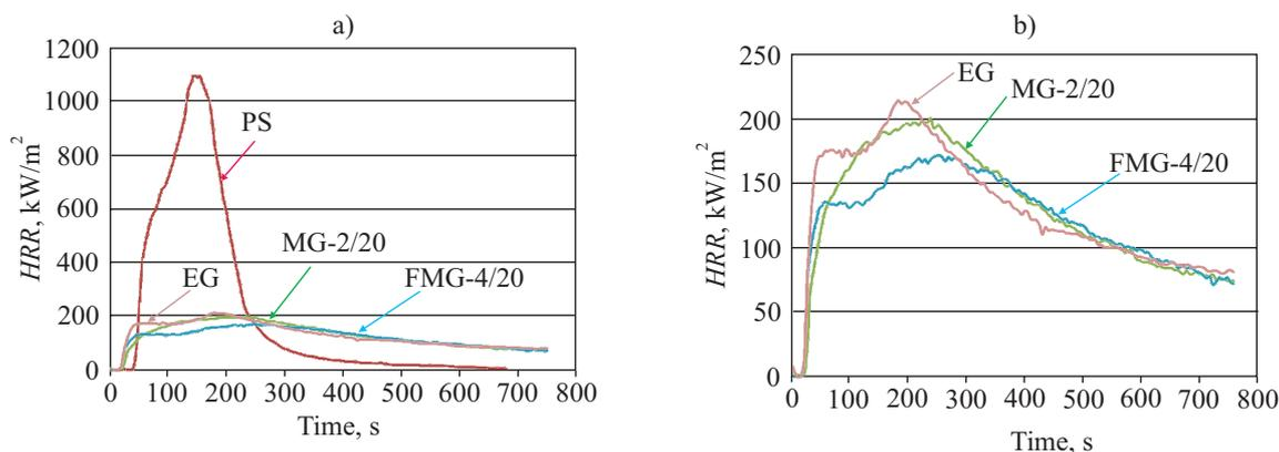
Fig. 2. Heat release rate per unit area as a function of time, with and without the control PS sample: PS — non-modified polystyrene, MG-2/20 — polystyrene with MG-2, FMG-4/20 — polystyrene with FMG-4, EG — polystyrene with expandable graphite
