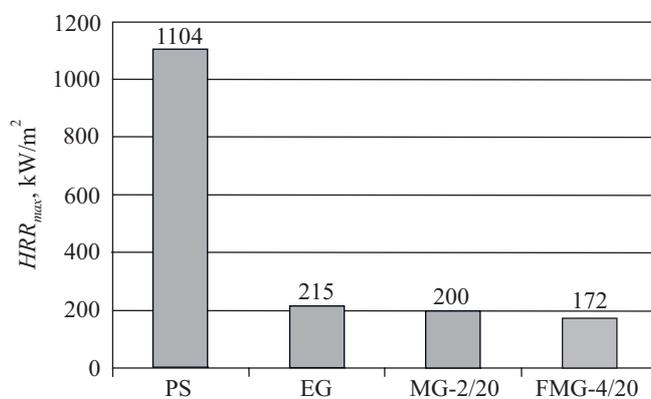
**Fig. 1. Maximum heat release rate per unit area, PS – non-modified polystyrene, EG – polystyrene with expandable graphite, MG-2/20 – polystyrene with MG-2, FMG-4/20 – polystyrene with FMG-4**
