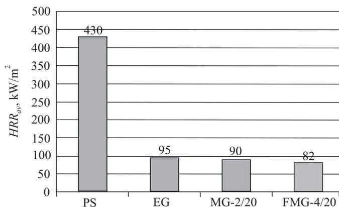
Fig. 3. Average heat release rate per unit area, PS — non-modified polystyrene, EG — polystyrene with expandable graphite, MG-2/20 — polystyrene with MG-2, FMG-4/20 — polystyrene with FMG-4
