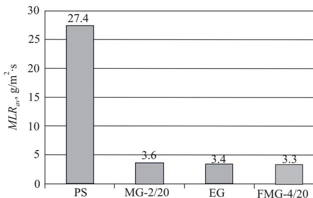
Fig. 5. Average mass loss rate, PS — non-modified polystyrene, FMG-4/20 — polystyrene with FMG-4, EG — polystyrene with expandable graphite, MG-2/20 — polystyrene with MG-2
