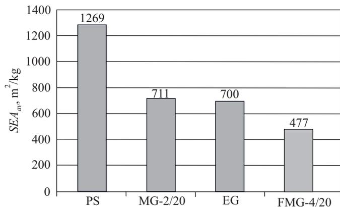
Fig. 4. Specific extinction area, PS — non-modified polystyrene, MG-2/20 — polystyrene with MG-2, EG — polystyrene with expandable graphite, FMG-4/20 — polystyrene with FMG-4
