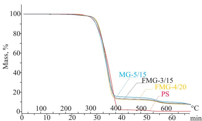
Fig. 6. Thermogravimetric analysis of PS with and without graphite additives
