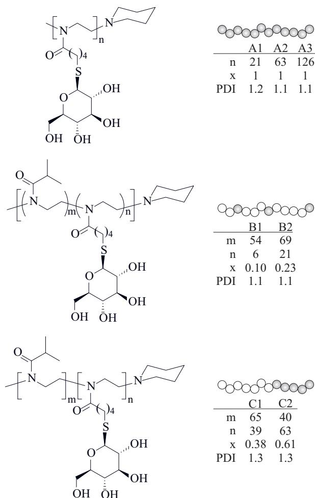
Scheme A. Chemical structures of glucopolyoxazoline homopolymers A1-3, statistical copolymers B1-2, and block copolymers C1-2;  $n$ ,  $m$ : number-average degrees of polymerization ( $^1\text{H}$  NMR),  $x = n/(m+n)$ : mole fraction of glucose units, PDI: apparent polydispersity index (SEC)
