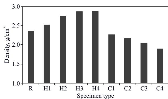
*Fig. 2. Effect of PC specimens composition on their unit weight*
