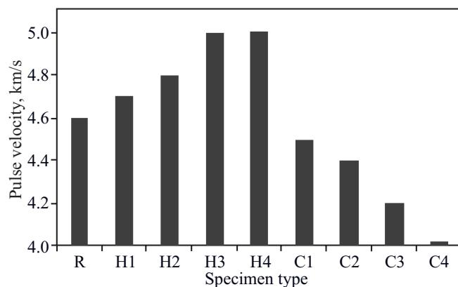
Fig. 3. Effect of PC specimens composition on their ultrasound pulse velocity
