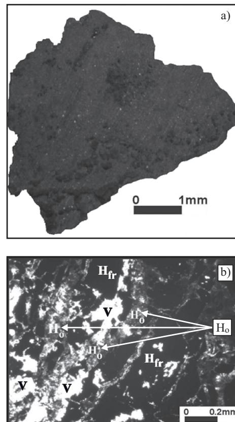
*Fig. 1. Mineralogical structure of hematite: a) general view of aggregate, b) structure of aggregate with oxide zones ( $H_O$ ), fresh zones ( $H_{fr}$ ) and voids (V)*
