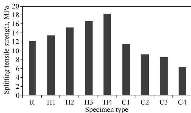
Fig. 6. Effect of PC specimens composition on their splitting tensile strength
