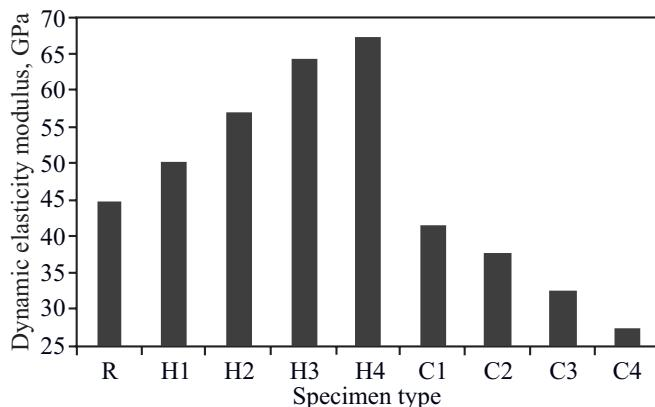
Fig. 8. Effect of PC specimens composition on their dynamic elasticity modulus
