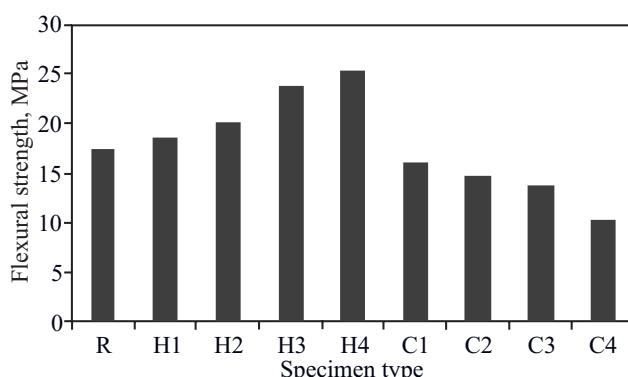
Fig. 5. Effect of PC specimens composition on their flexural strength
