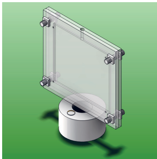
Fig. 2. Mold for foaming of TPUR and composites with CB
