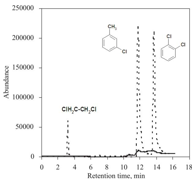
Fig. 2. Chromatograms of organochlorine compounds not adsorbed at temperature 200 °C in a microreactor filled with regenerated  $\text{Ag}/\text{Al}_2\text{O}_3$  (solid line) and pure  $\text{Al}_2\text{O}_3$  (dashed line)
