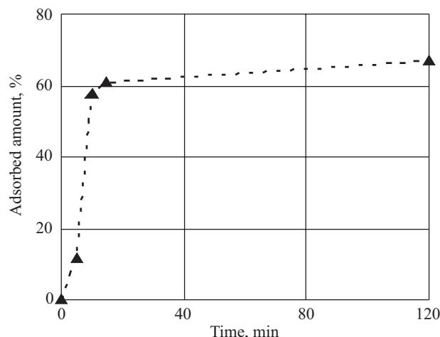
Fig. 1. Adsorption efficiency of 1,2-dichlorobenzene solved in mixture of Oil T110 and decalin (1:1 volume ratio) onto silver at temperature 150 °C as a function of time
