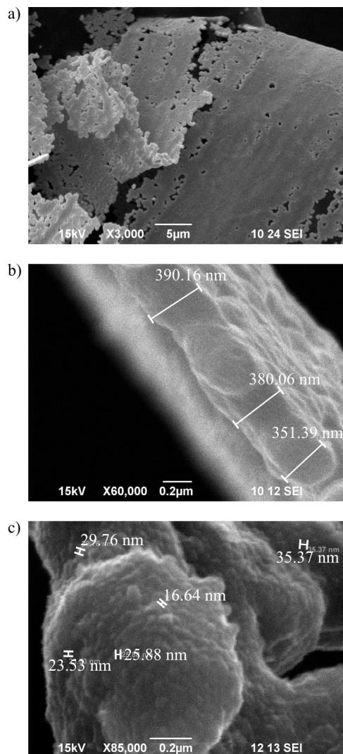
Fig. 1. The SEM image of the copper layer of thickness approximately 200–400 nm obtained by current pulse electrolysis with a reverse of the current direction at stainless cathode; SEM magnifications: a) 3000, b) 60 000, c) 85 000
