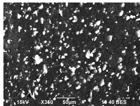
Fig. 2. The SEM image of a cross section of a PE-LD polymer composite with 30 wt. % of Cu flakes
