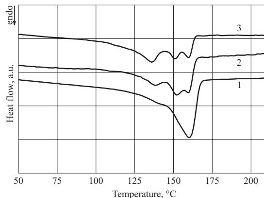
Fig. 3. DSC melting curves of composites aged in the accelerated way by xenon lamp irradiation for: 1 — 100 h, 2 — 200 h, 3 — 300 h; depth of removed sample 0.05 mm
