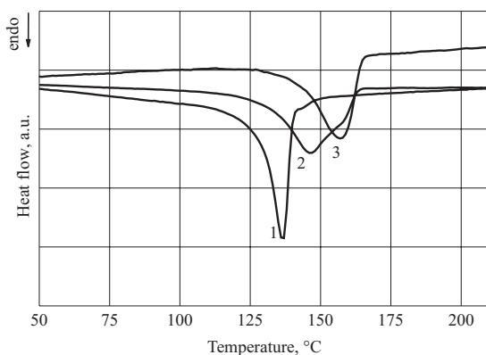
Fig. 2. DSC melting curves of the composite aged in atmosphere conditions: 1 — material not attached to the molding surface, 2 — material removed from the surface layer to the depth of about 0.05 mm, 3 — material removed from the deeper layer (from the depth between about 0.05 and 0.1 mm)
