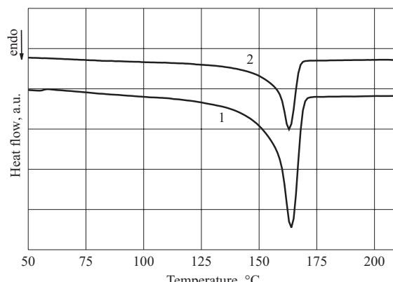
Fig. 1. DSC melting curves of: 1 – polypropylene Moplen HP548R, 2 – non-aged composite
