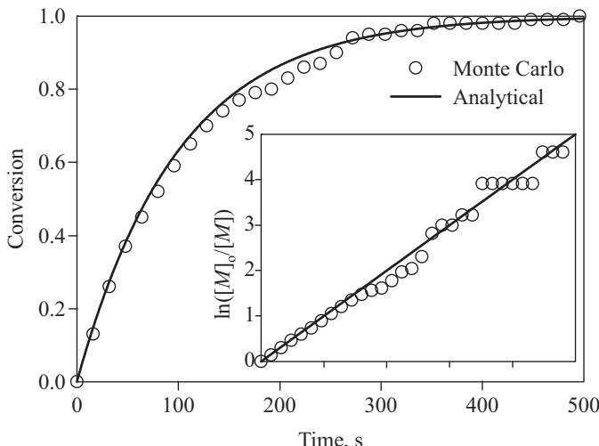
Fig. 2. An example of simulations of monomer conversion in a living/controlled homopolymerization with fast initiation. Conditions:  $n_{0M} = 100$ ,  $k_p = 1.0 \text{ l} \cdot \text{mol}^{-1} \cdot \text{s}^{-1}$ ,  $[M]_0 = 1.0 \text{ mol} \cdot \text{l}^{-1}$ , and  $[I]_0 = 0.01 \text{ mol} \cdot \text{l}^{-1}$ . The bottom axis for the semilogarithmic plot has the same range as that for the conversion plot
