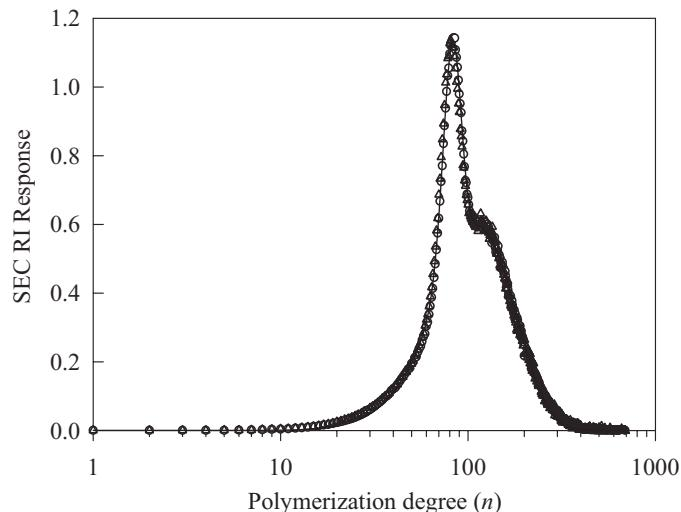
Fig. 9. Comparison of MWD obtained from Monte Carlo simulations and integration of differential equations. Triangles — the new Monte Carlo algorithm; circles — Monte Carlo algorithm proposed by Szymanski; line — integration of differential equations. Conditions described in the text
