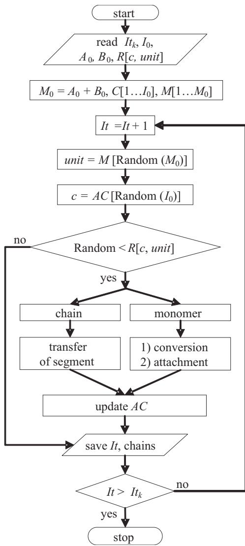
Fig. 8. Flowchart for modelling of monomer conversion, MWD, and microstructure of chains in copolymerization with segmental exchange
