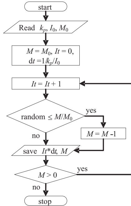
Fig. 1. Flowchart for modelling of monomer conversion in a living/controlled homopolymerization with fast initiation
