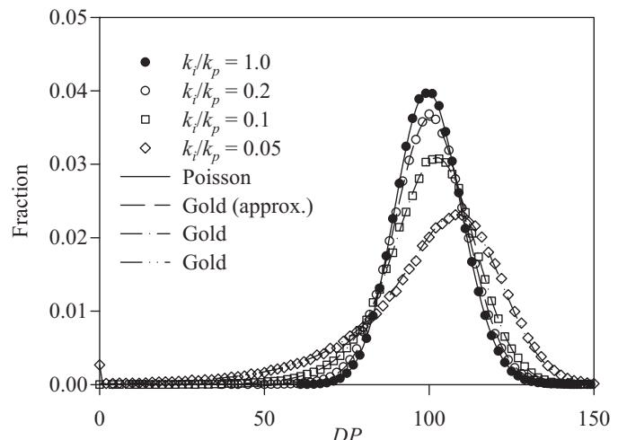
Fig. 5. Modelling of MWD in the living/controlled homopolymerization with slow initiation. Conditions:  $n_{0M} = 1 \cdot 10^7$ ,  $n_{0I} = 1 \cdot 10^5$ ,  $[M]_0 = 1.0 \text{ mol} \cdot \text{l}^{-1}$ ,  $[I]_0 = 0.01 \text{ mol} \cdot \text{l}^{-1}$ , and  $k_p = 1.0 \text{ l} \cdot \text{mol}^{-1} \cdot \text{s}^{-1}$ ;  $k_t$ : (●) 1.0, (○) 0.2, (□) 0.1, (◊) 0.5  $\text{l} \cdot \text{mol}^{-1} \cdot \text{s}^{-1}$ , respectively
