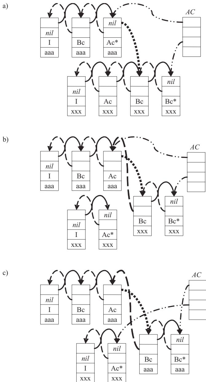
Fig. 7. Illustration of process of segment exchange between macromolecules: a) — attack of an active center on a monomeric unit randomly selected from the population, b) — breaking of bonds between the attacked monomeric unit and its predecessor, c) — connecting of attacked unit to a new host chain and updating pointers to new active centers
