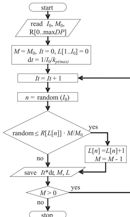
Fig. 3. Flowchart for modelling of monomer conversion and MWD in a living/controlled homopolymerization with slow initiation
