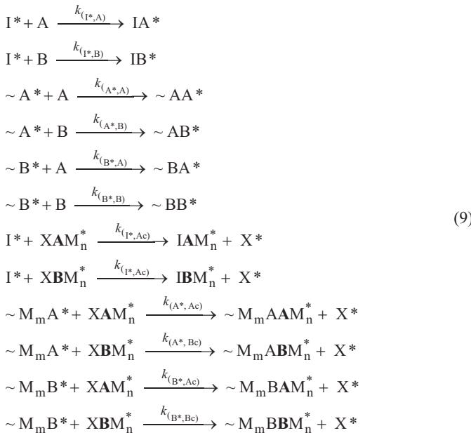
where:  $I, A, B$  — designate initiator and monomer molecules, respectively,  $X^*$  — stand for a chain fragment with active centers  $I^*, A^*$ , or  $B^*$ . Bolded characters mark monomeric units being an object of the attack.
