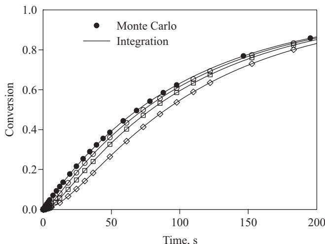
Fig. 4. Modelling of monomer conversion in a living/controlled homopolymerization with slow initiation. Conditions:  $n_{0M} = 1 \cdot 10^7$ ,  $n_{0I} = 1 \cdot 10^5$ ,  $[M]_0 = 1.0 \text{ mol} \cdot \text{l}^{-1}$ ,  $[I]_0 = 0.01 \text{ mol} \cdot \text{l}^{-1}$ , and  $k_p = 1.0 \text{ l} \cdot \text{mol}^{-1} \cdot \text{s}^{-1}$ .  $k_t$ : (●) 1.0, (○) 0.2, (□) 0.1, (◊) 0.5  $\text{l} \cdot \text{mol}^{-1} \cdot \text{s}^{-1}$ , respectively
