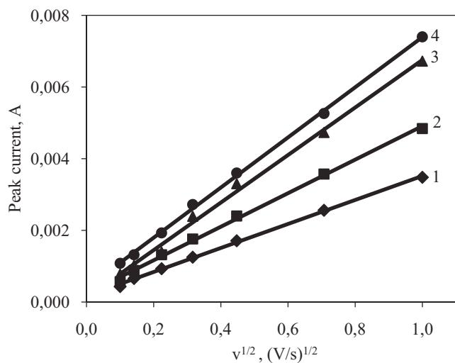
*Fig. 3. Dependence of the peak current in flavanone oxidation at Pt on the square root of the polarization rate ( $v$ ) for various flavanone solution concentrations ( $c$ ): 1 –  $2 \cdot 10^{-3}$  M, 2 –  $3 \cdot 10^{-3}$  M, 3 –  $4 \cdot 10^{-3}$  M, 4 –  $5 \cdot 10^{-3}$  M*
