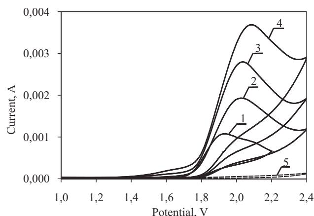
Fig. 2. Cyclic voltammograms of flavanone oxidation on the Pt electrode for  $5 \cdot 10^{-3}$  M flavanone solution in supporting electrolyte and for various polarization rates ( $v$ ): 1 –  $0.01$  V · s<sup>-1</sup>, 2 –  $0.05$  V · s<sup>-1</sup>, 3 –  $0.1$  V · s<sup>-1</sup>, 4 –  $0.2$  V · s<sup>-1</sup>; for comparison curve 5 – supporting electrolyte ( $v = 0.01$  V · s<sup>-1</sup>)
