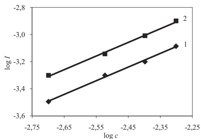
*Fig. 4. Dependence of the logarithm of oxidation current ( $I$ ) on the logarithm of flavanone concentration ( $c$ ) for polarization rate  $v = 0.01 \text{ V} \cdot \text{s}^{-1}$  at a constant electrode potential ( $E$ ) equal: 1 –  $1.85 \text{ V}$ , 2 –  $1.90 \text{ V}$*
