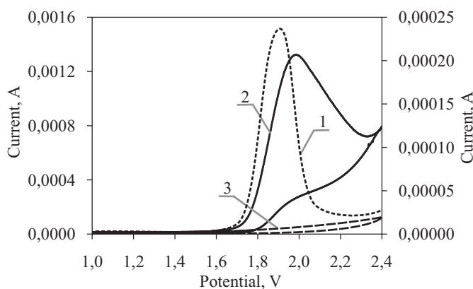
Fig. 1. Voltammograms of flavanone oxidation on the Pt electrode for  $5 \cdot 10^{-3}$  M flavanone solution in supporting electrolyte and polarization rate  $v = 0.01$  V · s<sup>-1</sup>: 1 – differential pulse curve (right axis), 2 – cyclic voltammogram (left axis); for comparison curve 3 – cyclic voltammogram of supporting electrolyte (left axis)
