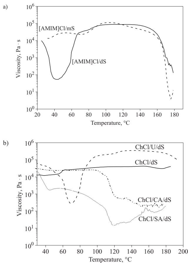
Fig. 1. Rheometric curves for ILs/starch systems with mass ratio 30:100: a) with [AMIM]Cl and dry starch (dS, 3 wt. % of water) or moist starch (mS, 14 wt. % of water); b) based on dry starch with ChCl itself or with deep eutectic mixtures of ChCl with urea (ChCl/U 1:2 mol/mol), citric acid (ChCl/CA 2:1 mol/mol) or succinic acid (ChCl/SA 1:1 mol/mol)
